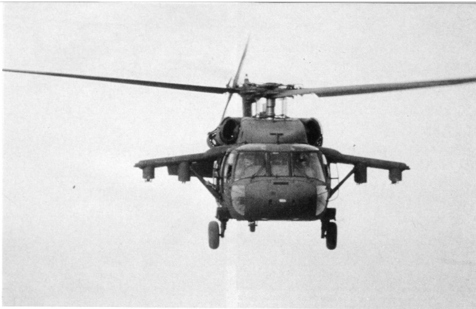
This U.S. Army UH-60 Blackhawk is equipped with ESSS bolt-on stub wings. These wings are capable of mounting external fuel tanks and/or Hellfire anti-tank guided missiles. The Blackhawk also mounts two M60 machine guns, one on each side.
