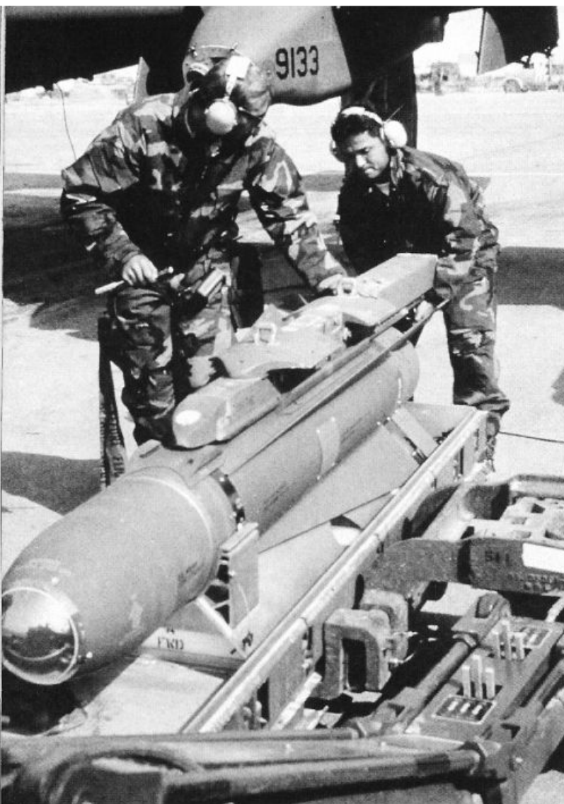
Armorers load Cluster Bomb Units on a Triple Ejector Rack. The TER can hold three CBUs, one on each side and one on the bottom.
