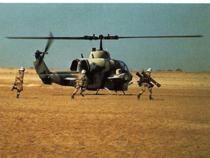
(Left) Marine ground crewmen rush to rearm a Bell AH-1W SuperCobra with TOW anti-tank missiles during DESERT STORM combat operations. Most Marine SuperCobras carried four to eight TOWs and 2.75 inch rocket pods.
