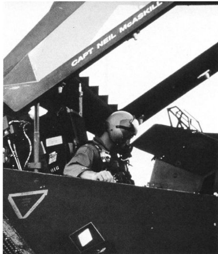
Stealth Fighter technology includes special coatings on the windscreen to deflect radar beams which would otherwise reflect off of the pilot and ejection seat. Other stealth features include radar absorbing paint, the faceting of the fuselage and wing, and shielded intakes and exhaust.
