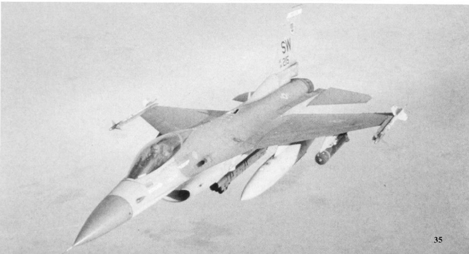
An F-16C of the 17th TFS, 363rd TFW lines up to take on fuel enroute to Iraq. It is armed with a CBU-87 and carries an AN/ALQ-119 jamming pod. This pod suffered a high rate of failure initially (one crew chief painted Black pods on his F-16 every time a pod failed) but as experience with the pods built up their reliability increased.
