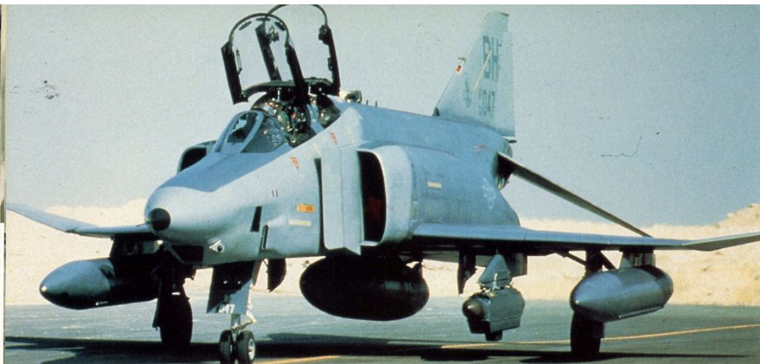
An RF-4C of the 117th TRG, Alabama ANG taxis in after a mission. Bulges on either side of the nose camera window are for Radar Homing and Warning (RHAW) antenna. The aircraft carries a jammer pod under the inboard wing pylon.
