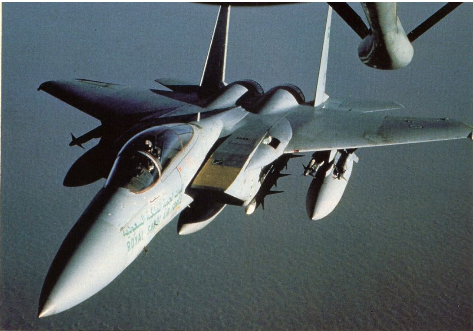
An F-15C Eagle of the Royal Saudi Air Force refuels over the Gulf during a DESERT STORM combat air patrol mission. The Eagle carries an air superiority weapons load of four AIM-7 Sparrows on fuselage stations and four AIM-9 Sidewinders on the wing pylons. To extend its time on station, the aircraft carries 610 gallon external fuel tanks on the fuselage centerline and under wing pylons.
