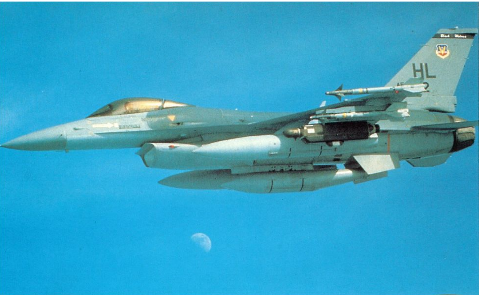
An F-16 of the 388th TFW enroute to Saudi Arabia as part of Operation DESERT SHIELD from Hill AFB, Utah. They are configured for long range and/or air defense with four Sidewinders and AN/ALQ-131 jamming pods. (USAF by TSGT Marvin D. Lynchard)
