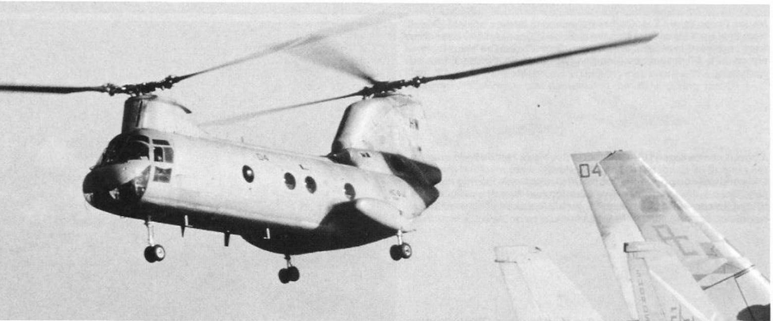
A Navy CH-46E Sea Knight of HC-5 shuttles supplies from USS SYLVANIA to USS JOHN F. KENNEDY on 21 January 1991. Sea Knights are the primary vert-rep (vertical replenishment) helicopter in service with the composite helicopter squadrons. (USCG by PA1 Chuck Kalnbach)
