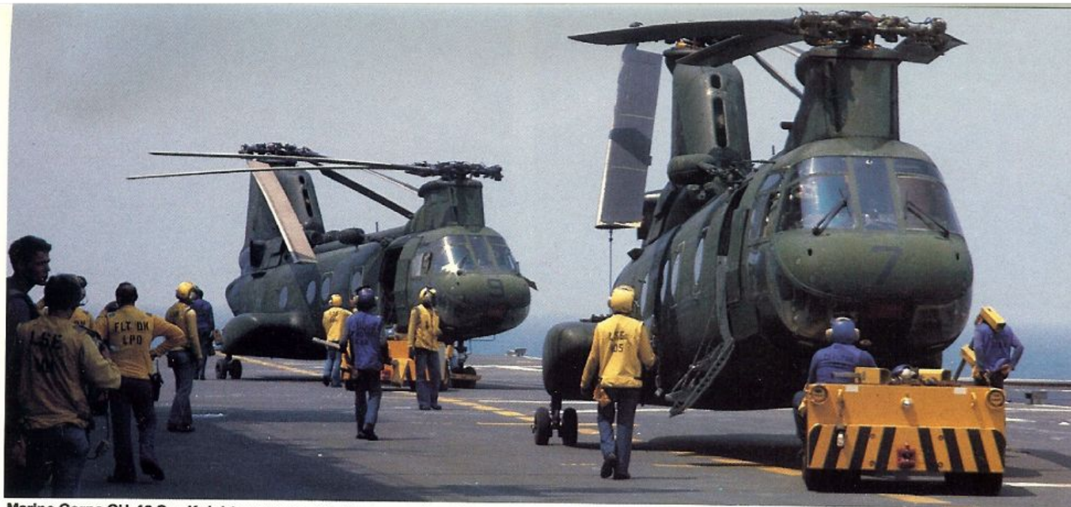
Marine Corps CH-46 Sea Knights were used to fly men and equipment from the LHA/LPH assault ships to airfields in Saudi Arabia. Later they were repainted in a Sand and Brown camouflage. The aircraft were armed with .50 caliber machine guns in the cabin windows, one on each side.
