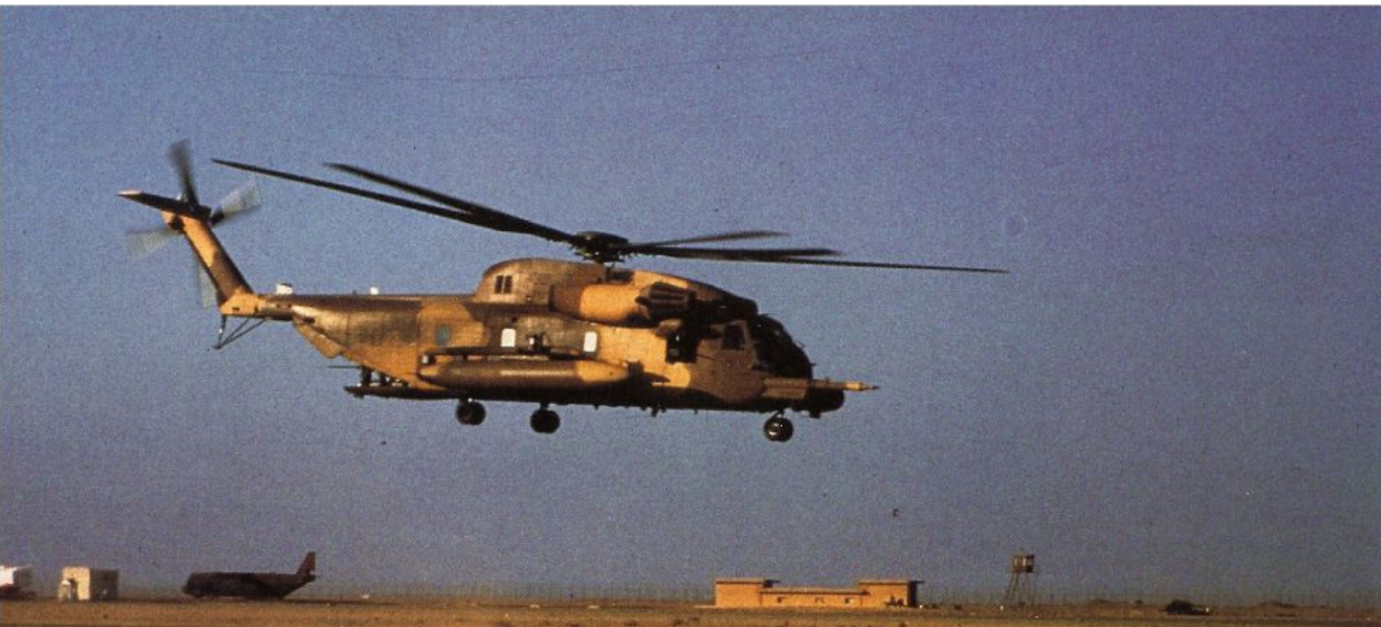
The MH-53J Pave Low Enhanced Super Jolly Green Giant rescue helicopter provided long range rescue capability for crews downed behind enemy lines. The MH-53J is equipped with an inertial navigation system, stabilized FLIR, Doppler navigation equipment, radar from an A-7D Corsair II and a computer projected moving map display. The first of the improved Jolly Greens was delivered to the USAF during 1987.
