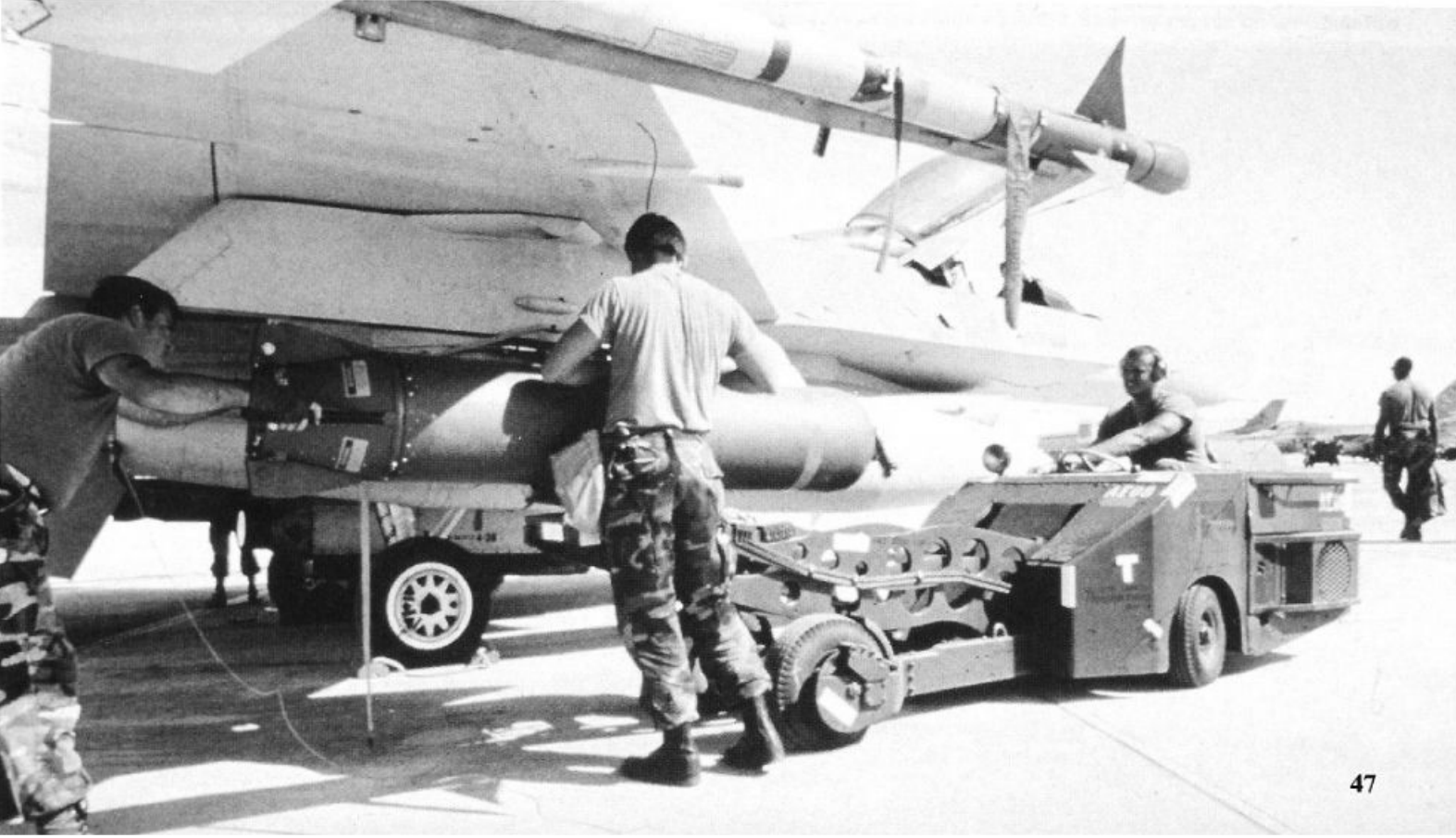
Armorerers load a CBU-87 on an F-16. The cluster bomb unit (CBU) is based on a common dispenser which can be loaded with various submunitions. The CBU-87/B dispenser deploys tail fins upon release which cause the bomb to spin. At a pre-set altitude, the case splits apart and 202 CBU-97/B bomblets are discharged.
