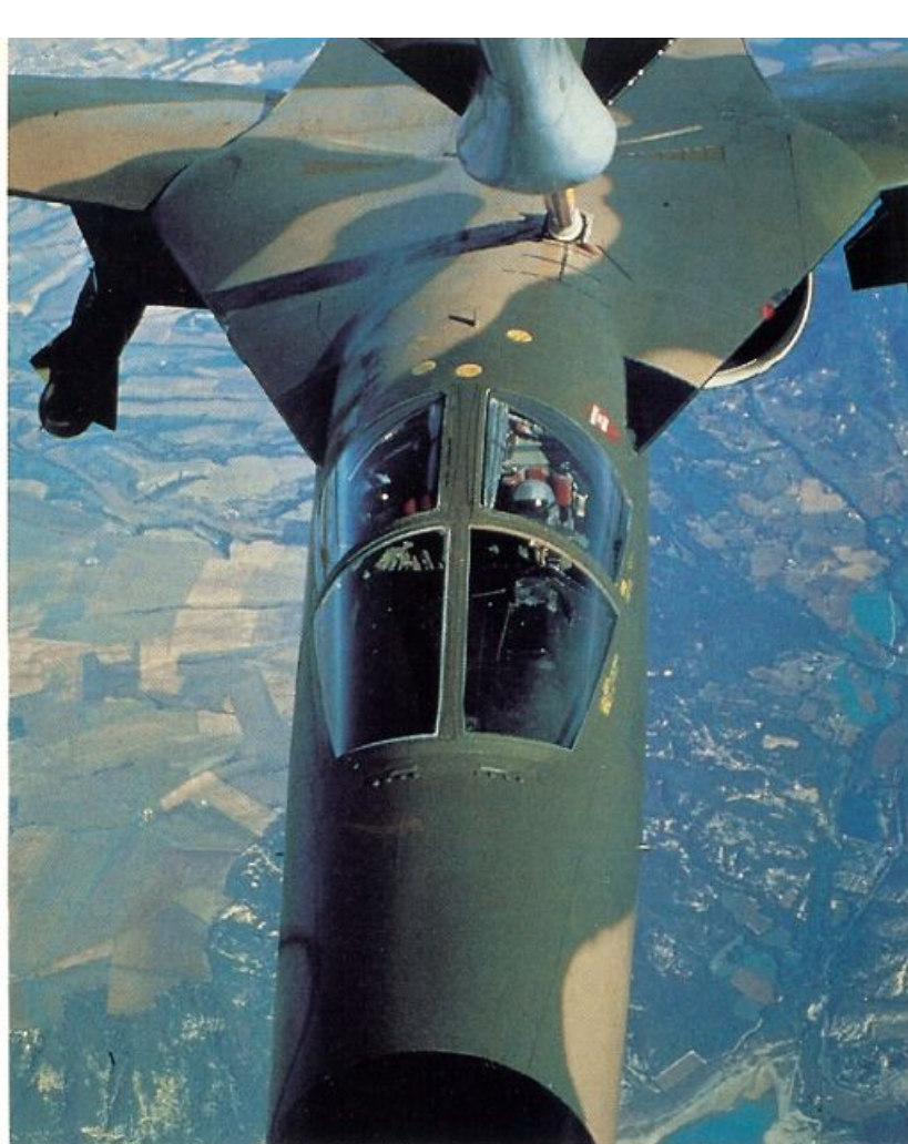
An F-111F of the 48th Tactical Fighter Wing, RAF Lakenheath, England refuels enroute to attack an Iraqi target. It is armed with a pair of GBU-15 electro-optical "smart" bombs which will be guided to the target by the AN/AVG-26 Pave Tack laser designator carried on the forward center-line fuselage station.
