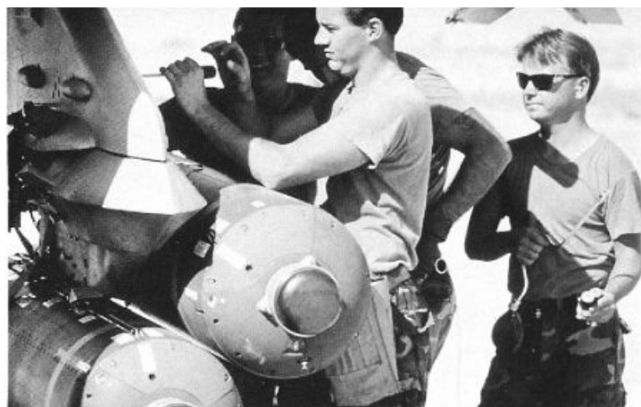
Armorers load Cluster Bomb Units on a Triple Ejector Rack. The TER can hold three CBUs, one on each side and one on the bottom.
