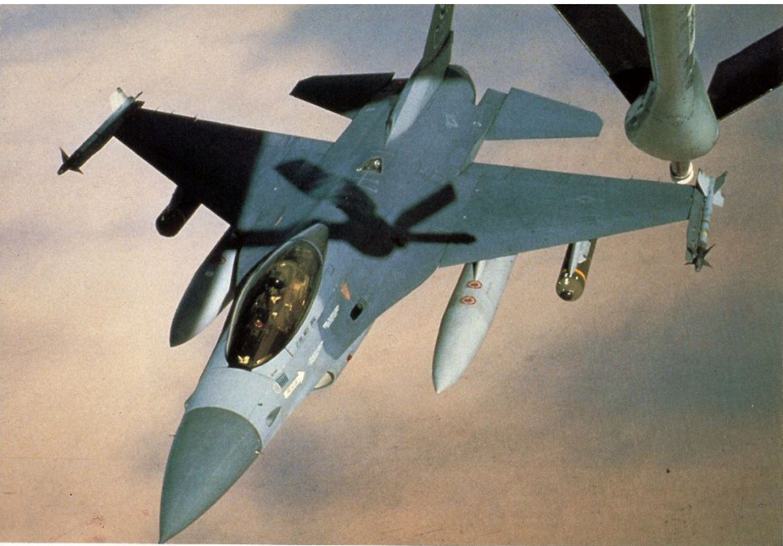
An F-16C Fighting Falcon of the 17th Tactical Fighter Squadron, 363rd Tactical Fighter Wing enroute to bomb the Iraqi Republican Guards in Kuwait. It is armed with Cluster Bomb Units, AIM-9 Sidewinder air-to-air missiles for self defense, and carried external fuel tanks. The pilot has started a mission scorecard under the canopy. (USAF by TSGT Perry Heimer)
