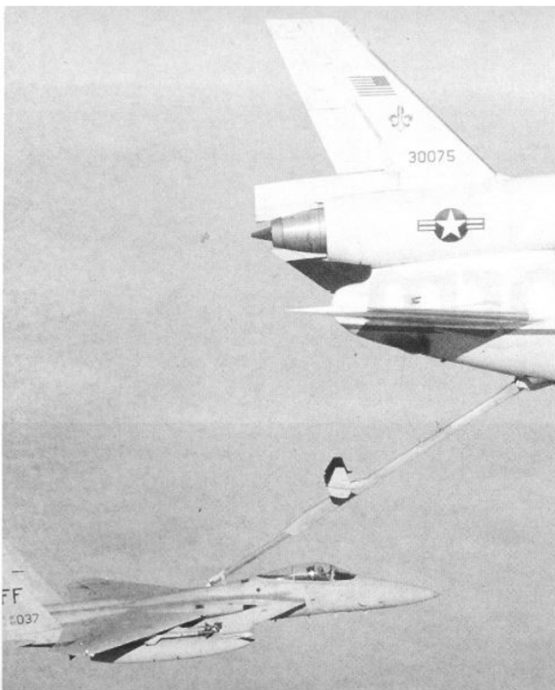
F-15s of the 27th Tactical Fighter Squadron, 1st Tactical Fighter Wing deployed from Langley Air Force Base, Virginia, to Saudi Arabia in some fourteen hours. The Eagles refueled at least eight times, usually from KC-10 Extenders. The Eagle was designed as a pure air superiority fighter and is a big aircraft, with a wingspan of forty-three feet and length of sixty-four feet. The F-15C has a maximum takeoff weight of 68,470 pounds.
