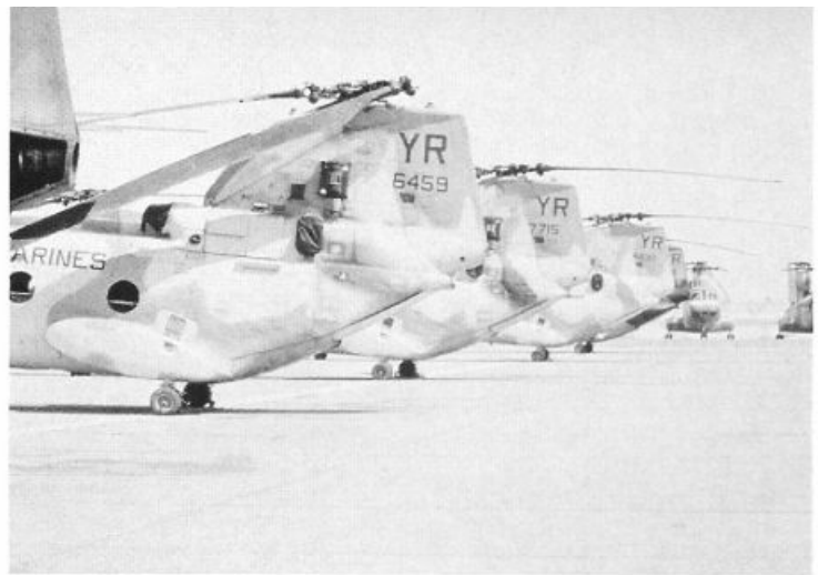
The Boeing Vertol CH-46 carries a crew of three and is capable of lifting 4,000 pounds of cargo. Different variants of the Sea Knight have been in service with the Navy and Marines since the early 1960s.
