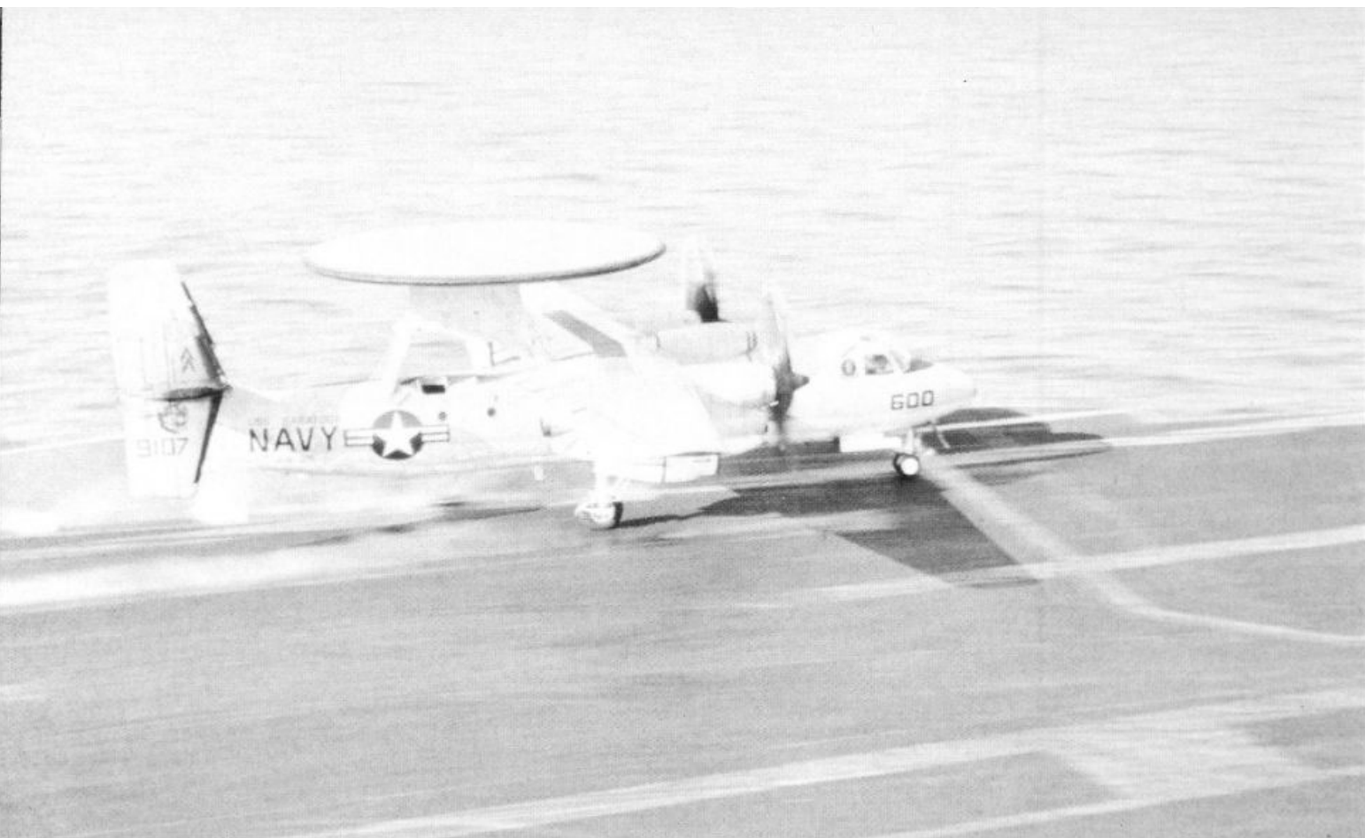
A Grumman E-2C Hawkeye of VAW-125 launches from the number four catapult aboard USS SARATOGA. Though a veteran of nearly 30 years of service, the E-2 continues to be the Navy version of the AWACS, providing early warning and air control for the fleet.
