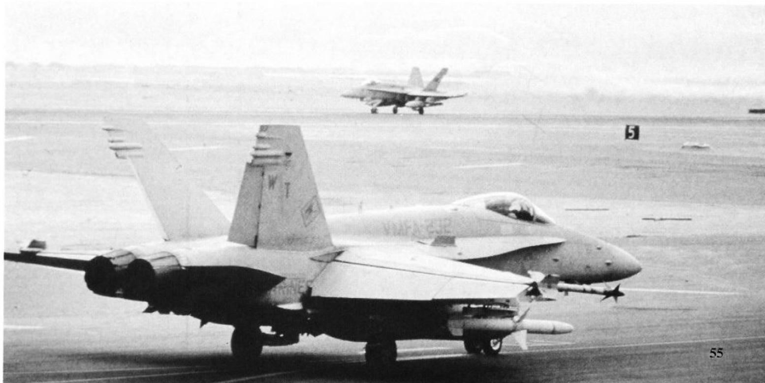
A Marine Corps F/A-18C Hornet of VMFA-232 Red Devils (based at MCAS Kaneohe Bay, Hawaii) taxis out for a DESERT STORM mission armed with HARM anti-radiation missiles on the wing pylons and Side-winders on the wingtips.
