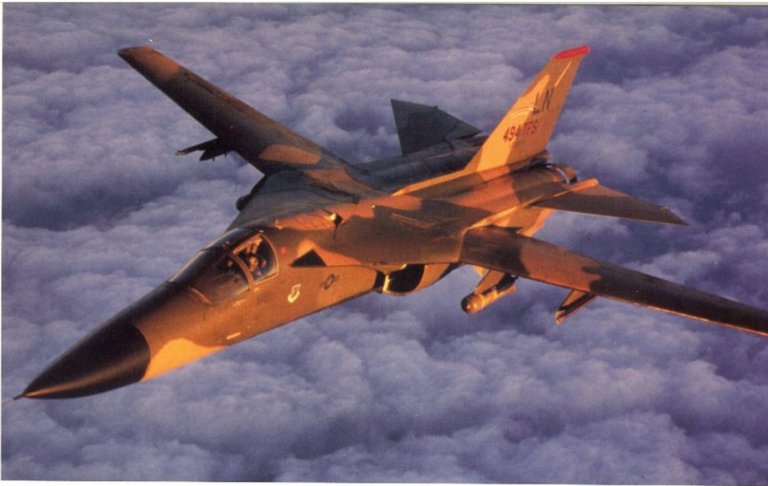
An F-111F of the 494th TFS, 48th TFW after a mission over Iraq. It is carrying a Cluster Bomb Unit on the inboard pylon. F-111s did much of their bombing against strategic targets deep inside Iraq, using their all-weather capabilities.
