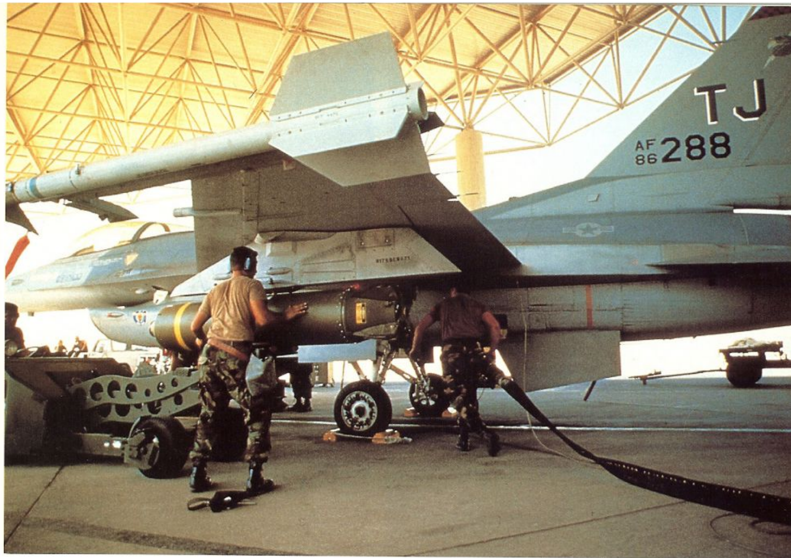
Ground crews refuel and rearm an F-16 of the 401st Tactical Fighter Wing. The aircraft carries Cluster Bomb Units on the wing pylon and an AIM-9L Sidewinder on the wingtip launcher. The Sidewinder is in Light Gray rather than the usual overall White.
