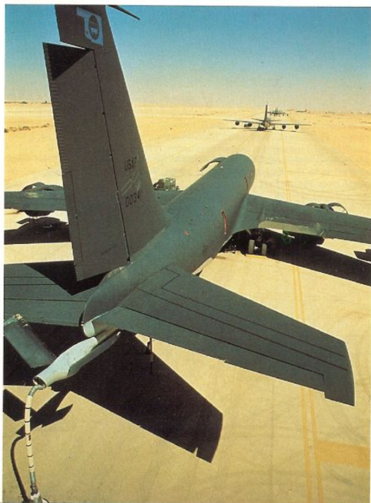
SAC KC-135s line up on the taxiway prepared to take off on a refueling mission with Navy and/or Marine aircraft as is evidenced by the drogue and basket attached to the refueling boom. While USAF aircraft are equipped with female refueling receptacles, Navy and Marine aircraft employ the probe and drogue method of refueling. The pace of DESERT STORM missions required supplementing Navy and Marine refueling assets with USAF tankers.
