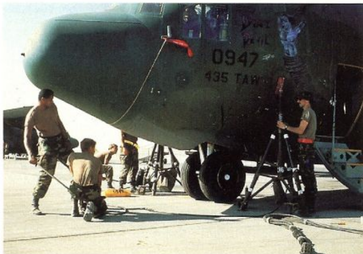
Maintenance troops prepare to change a tire on Dust Devil , a Lockheed C-130E Hercules of the 435th Tactical Airlift Wing.
