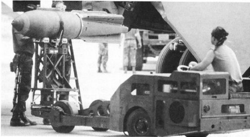
An Ordnance crew loads a 2,000 pound Mk 84 bomb onto an F-16. A lot was made of the difference between "smart" bombs and "dumb" bombs, ignoring the fact that ballistics computers in aircraft such as the F-16 and F/A-18 give the pilot the ability to place free-fall iron bombs on target with great accuracy.
