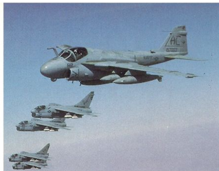
A-6E Intruders of VA-75 and Rockeye armed A-7Es of VA-46 Clansmen take up position to take on fuel from a KC-135 on 6 February 1991. The A-6E refueled first, then provided tanker service, using the centerline buddy pod, for some of the A-7s. (USAF by TSGT Rose Reynolds)
