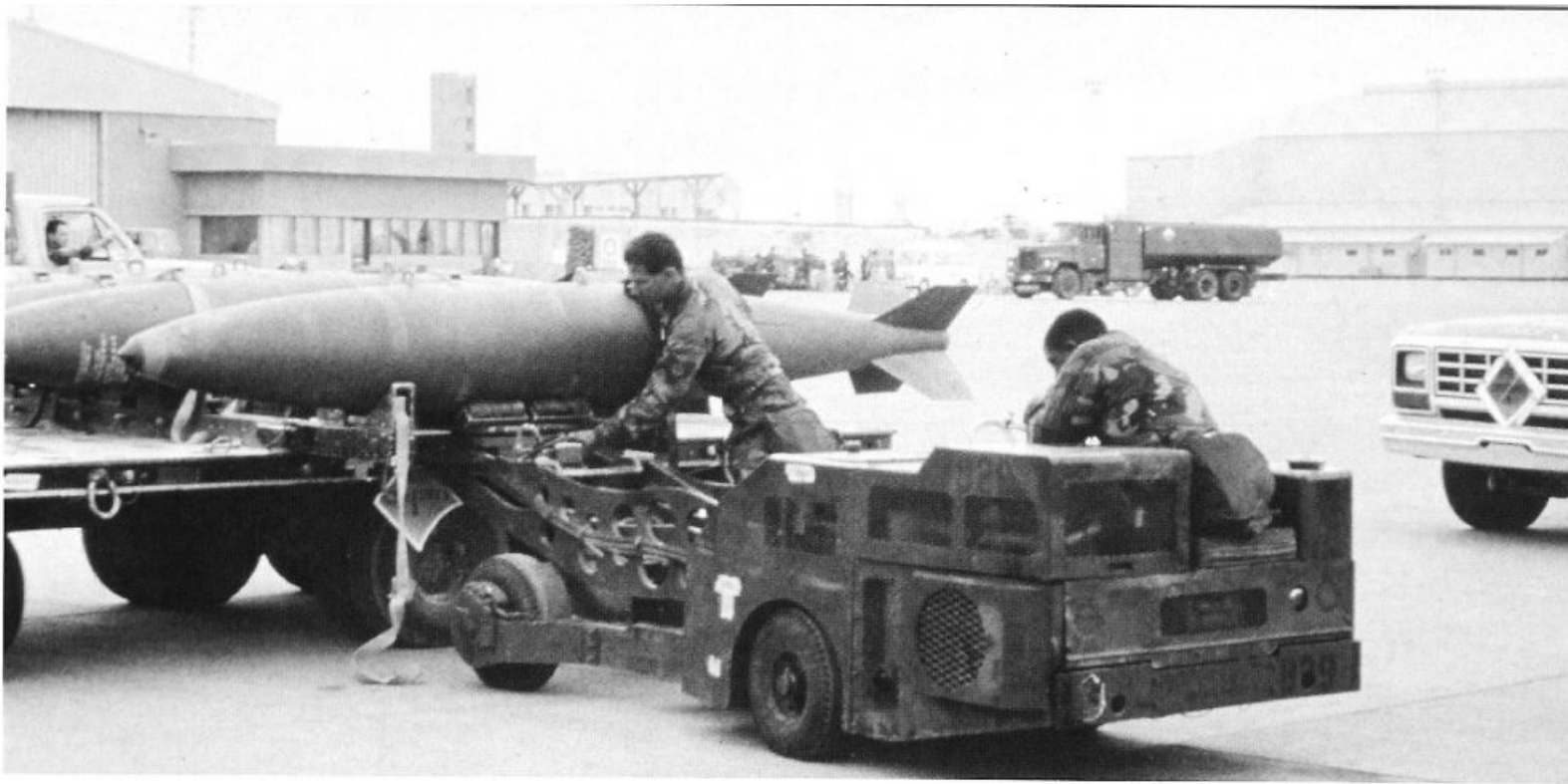
An Ordnance crew loads a 2,000 pound Mk 84 bomb onto an F-16. A lot was made of the difference between "smart" bombs and "dumb" bombs, ignoring the fact that ballistics computers in aircraft such as the F-16 and F/A-18 give the pilot the ability to place free-fall iron bombs on target with great accuracy.
