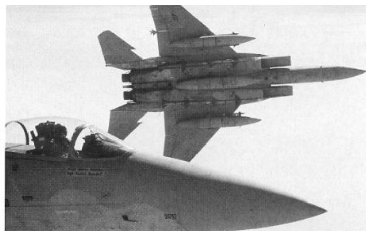
An F-15C Eagle of the 1st Tactical Fighter Wing peels off, heading for a target in Iraq. The aircraft is armed with four AIM-7F Sparrows and four AIM-9 Sidewinder air-to-air missiles and carries three drop tanks.
