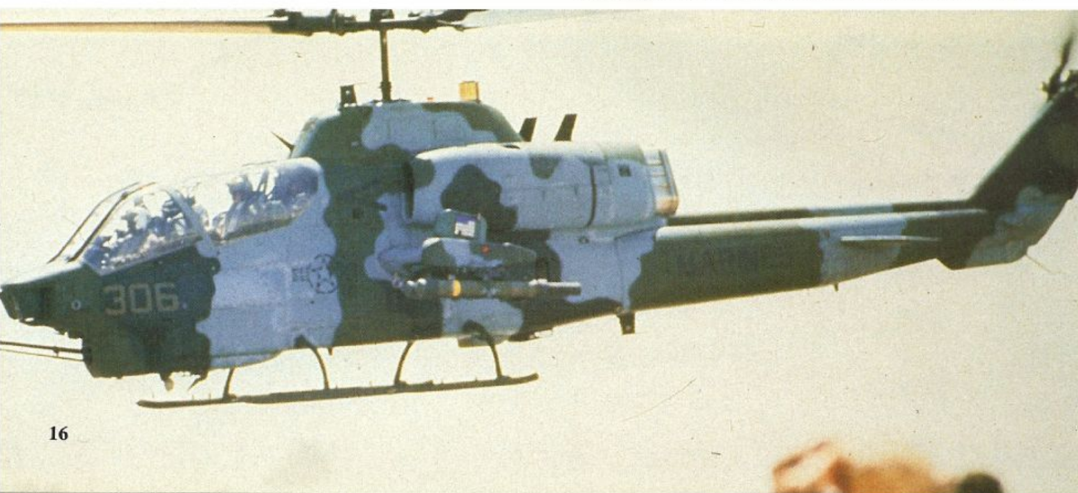
A Hellfire missile armed Marine AH-1W SuperCobra takes off for a ground support mission during DESERT STORM. For countermeasures, the AH-1Ws were equipped with chaff/flare launchers on the stub wings and a DISCO light IR jammer behind the main rotor.
