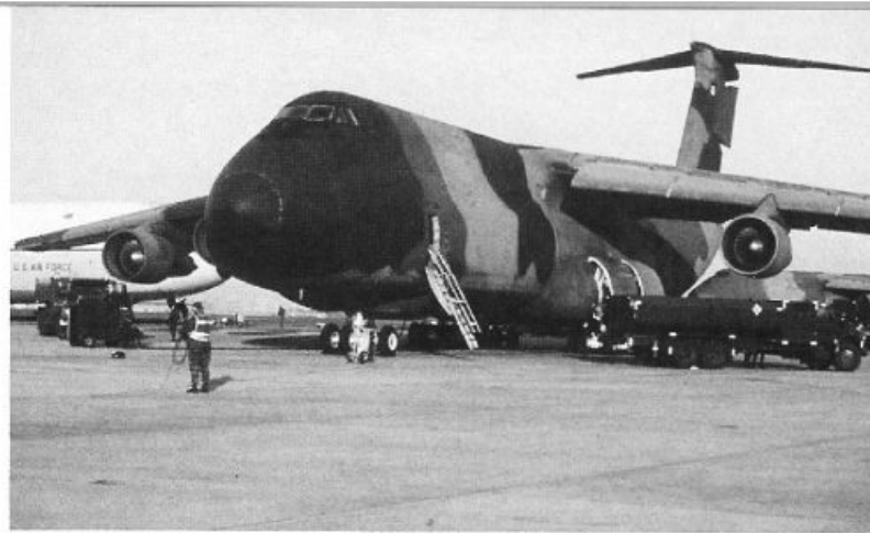
The world-champion airlifter is the gigantic Lockheed C-5A Galaxy, which has a gross takeoff weight in excess of 764,000 pounds. 435th TAW fuels personnel refuel a C-5 on the ramp at Rhein Main Air Base, Germany prior to a resupply flight to the Persian Gulf. The USAF lost one C-5 on a mission from Germany to the Gulf. (USAF by SRA Michael Eyer)
