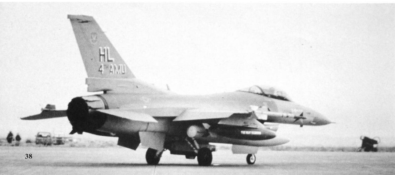
An F-16C of the 4th TFS, 388th TFW. The C model incorporated several advances in avionics over the A model, including a Westinghouse APG-68 multi-mode radar, new cockpit displays, a GEC Avionics wide angle head-up-display (HUD) with forward-looking infrared (FLIR) video and increased memory for its mission computers.
