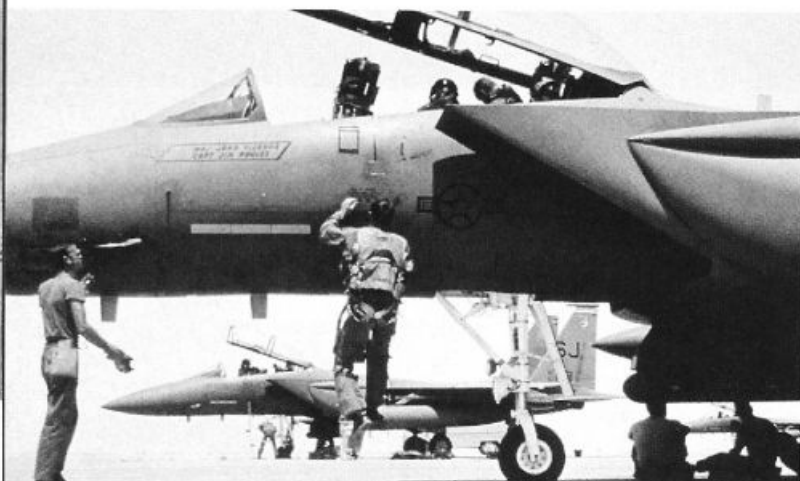
A Strike Eagle pilot climbs on board his F-15E for a DESERT STORM sortie. The aircraft is equipped with conformal fuel tanks, known as Fast Packs. The aircraft is overall Gun Gray. The Air Force lost two F-15Es during DESERT STORM, both during the first days of the war.
