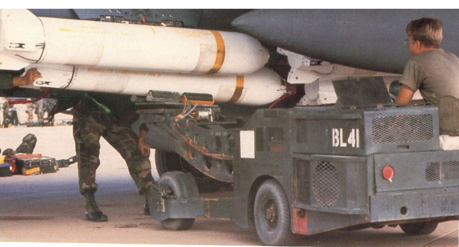
Ground crews load MK-20 Rockeye CBUs on an F-15E Strike Eagle of the 4th TFW. The MK-20 Rockeye is one of the most widely used CBUs and was first used in the Vietnam War. It weighs 490 pounds and contains 247 M-118 bomblets which are released at an altitude of 500 feet, covering an area of 30,000 square feet.
