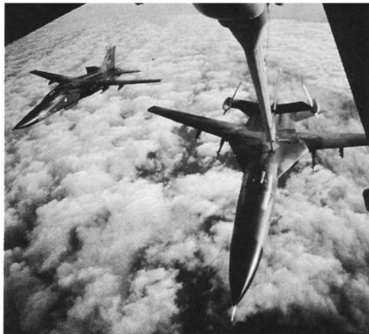
48th TFW F-111s are refueled by a KC-10 Extender. The official USAF caption states that they are returning from their first combat missions over Iraq and Kuwait. They are armed with AIM-9 Sidewinders on the inboard pylons and carry ALQ-131 jamming pods under the forward fuselage. (USAF by SRA Chris Putman)
