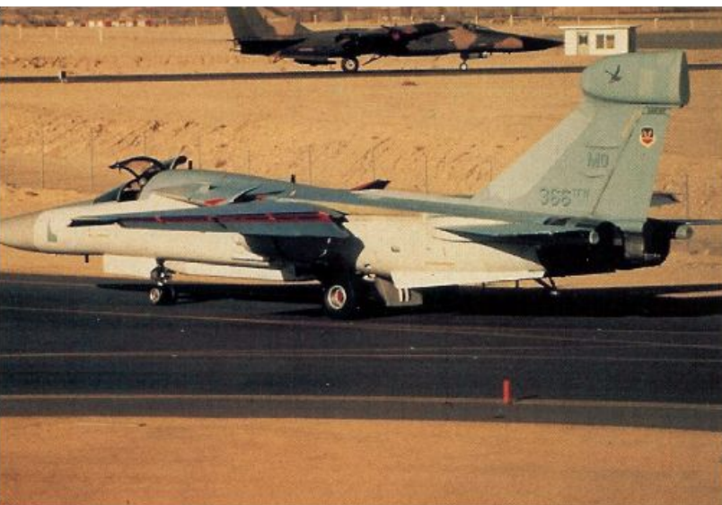
An EF-111F Raven taxis out for a mission over Iraq. EF-111s escorted strike groups of F-111F bombers providing jamming support against air defense radars.
