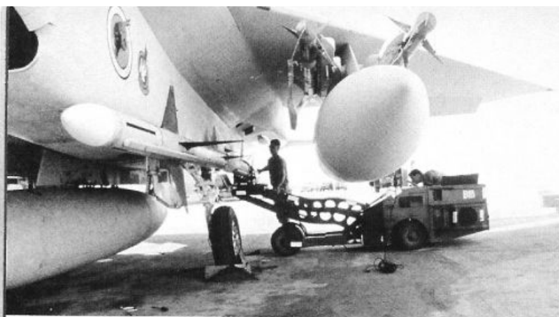
Ground crewmen load AIM-7 Sparrow air-to-air missiles on the fuselage stations of an F-15C Eagle. The AIM-7 is an 'all aspect' radar guided missile, which means that it can be fired from any angle. The missiles on the wing pylon are AIM-9 Sidewinder infrared guided missiles.
