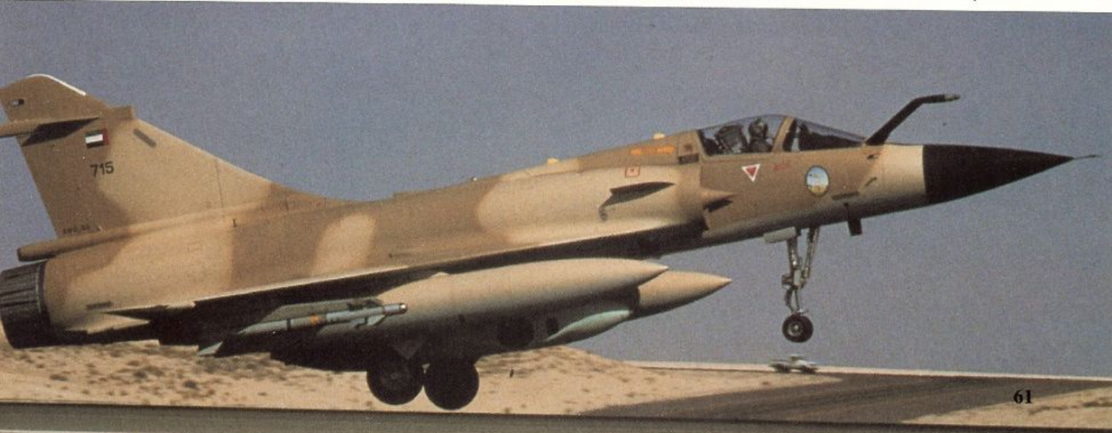
A United Arab Emirates Air Force Mirage 2000 air defense fighter takes off on a combat air patrol mission. The aircraft carries a Matra Magic AAM on the outboard pylon. (USAF by TSGT Perry Heimer)
