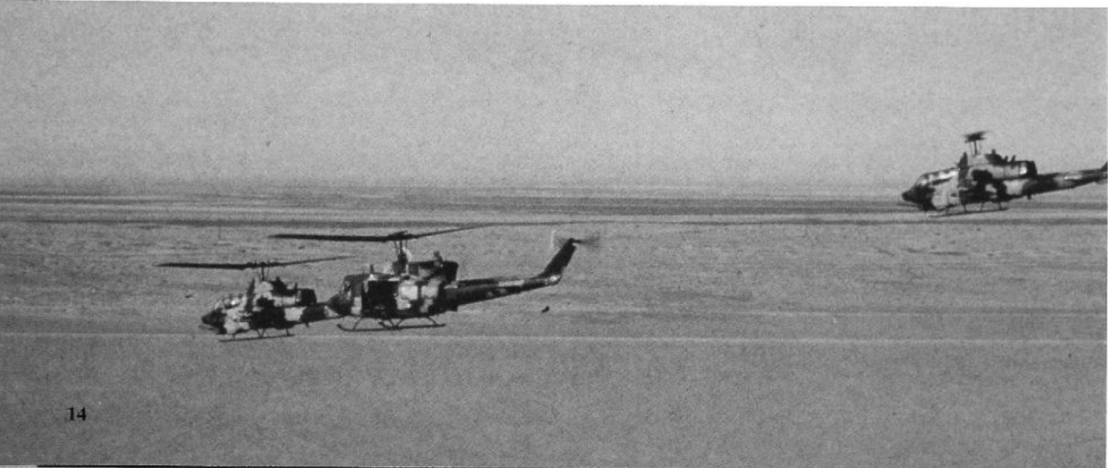
A pair of Marine AH-1W SuperCobras escort a UH-1N Huey on a reconnaissance mission over their Area of Operations. The SuperCobra is the latest AH-1 Cobra variant which was originally introduced during the Vietnam War (AH-1G). The AH-1W is powered by two 1,723 shp T700-GE-401 engines.
