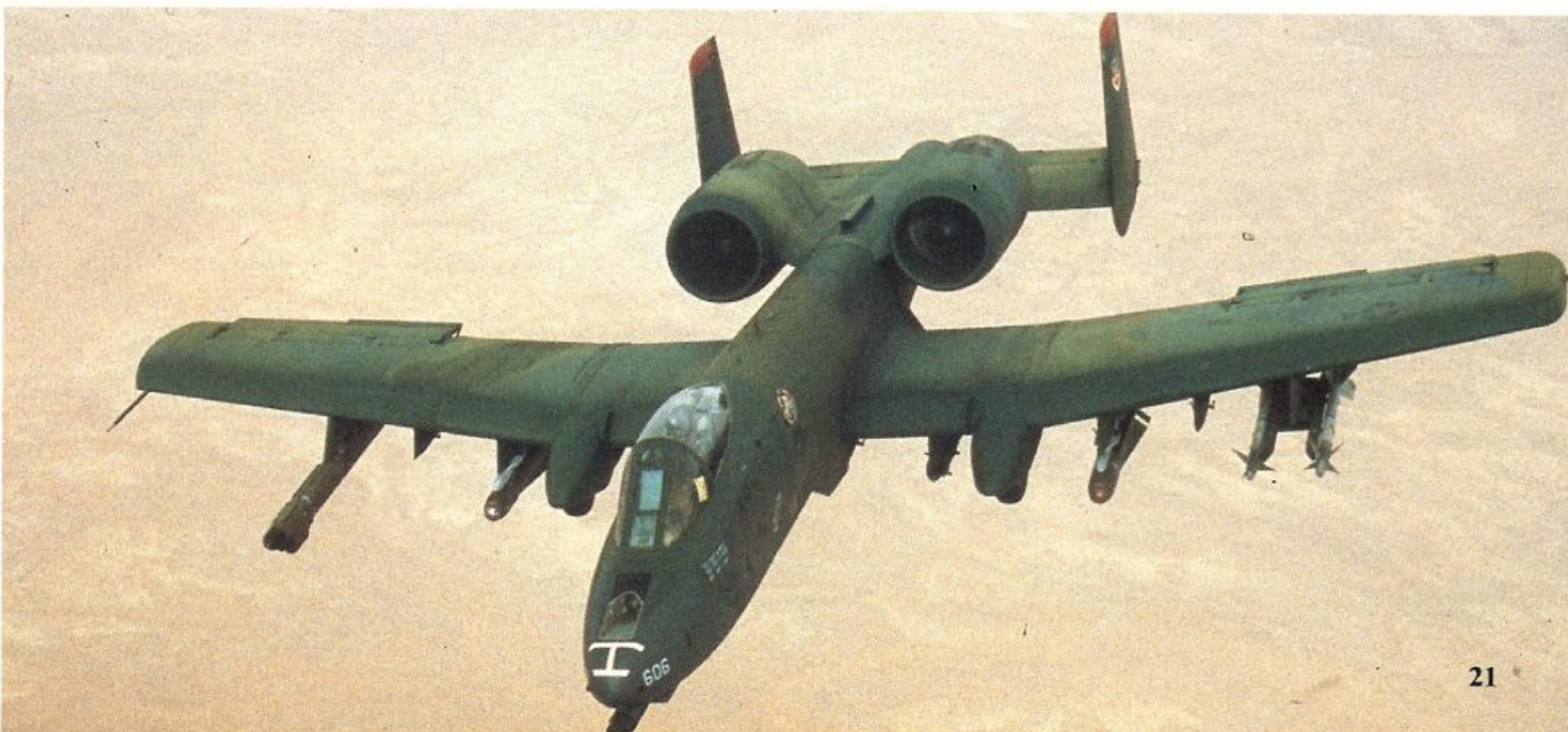
A-10A Thunderbolt II (Warthog) attack aircraft of the 23rd TFW, England AFB, Louisiana, the 354th TFW, Myrtle Beach AFB, South Carolina and the 10th TFW, RAF Lakenheath, England deployed to Saudi Arabia for DESERT STORM. The A-10 has been affectionately dubbed the Warthog by its pilots. This A-10 is armed with a pair of Maverick missiles and a pair of AIM-9 Sidewinder as it moves into position to take on fuel on 3 February 1991. (USAF by TSGT Rose Reynolds)
