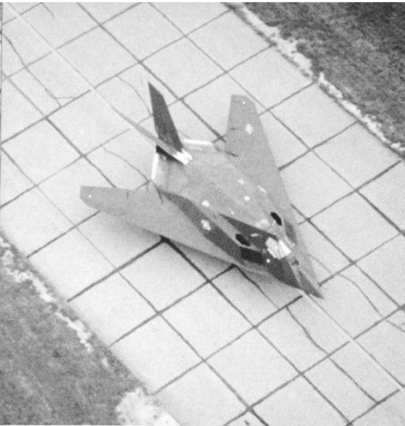
A Lockheed F-117A Stealth Fighter of the 37th TFW, based at the Tonopah Test Range, Nevada, taxis at Langley AFB prior to the unit's departure for Saudi Arabia and Operation DESERT SHIELD. The open auxiliary suck-in doors, just behind the intakes, provide additional air for taxiing and are closed during flight. (USAF MSGT Belcher)
